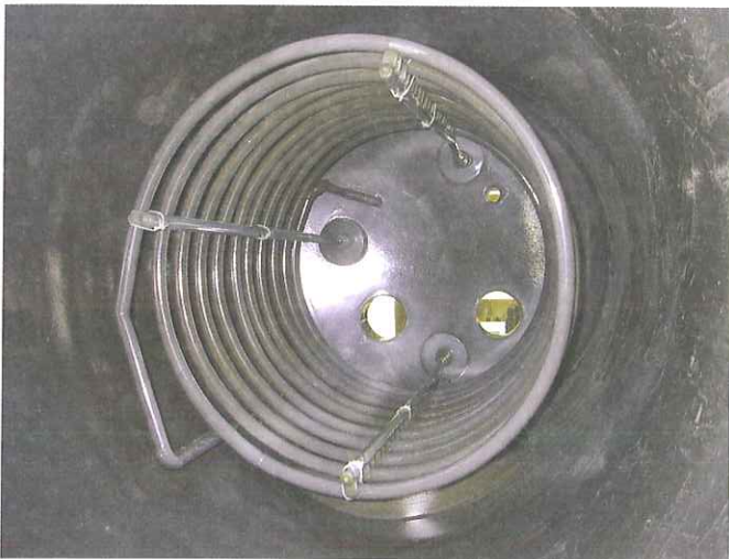
Application of the layer also on difficult to access or complex geometries, e.g. reaction tanks with coated heating coils.
