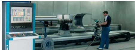
Set-up of the K2 system for carbide coating of the rollers
