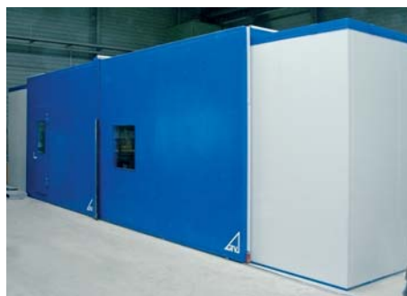
Overview of the system with sound insulation cabin, maximum component length 10 m
